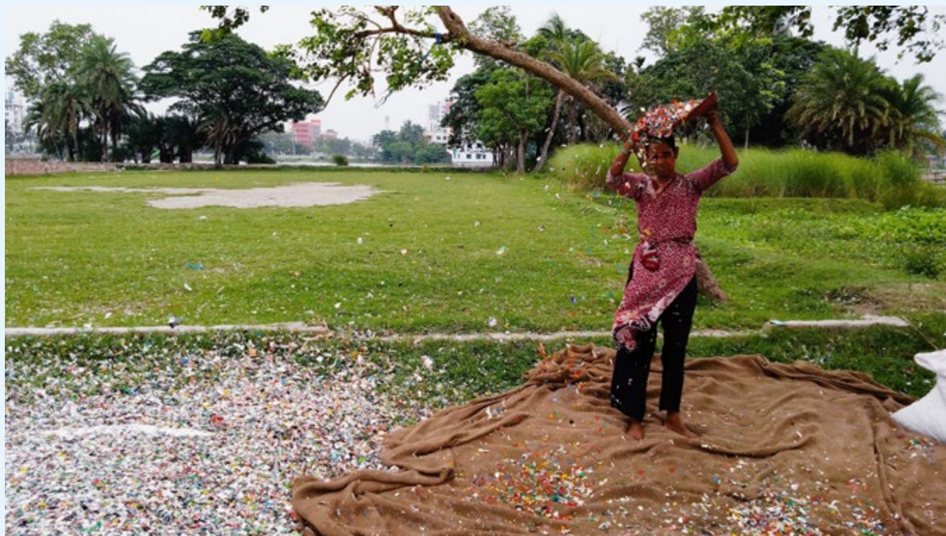
Figure 17: Manual plastic separation by wind. Photo by Philipp Lorber, 2023.
