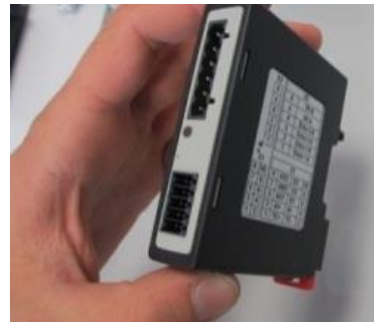
Fig. 11: Removing the controller module - part 2 (similar to picture)
