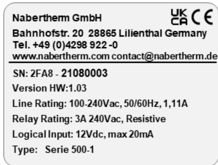
Fig. 7: Example (type plate of the control unit)
