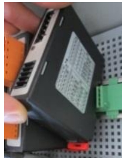
Fig. 11: Removing the controller module - part 2 (similar to picture)
